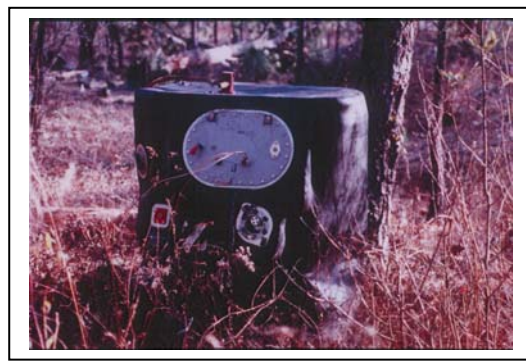
Figure 9. Missing fuel cell from AH-64 shown in figure 8. The cell was found full without any evidence of leakage.
