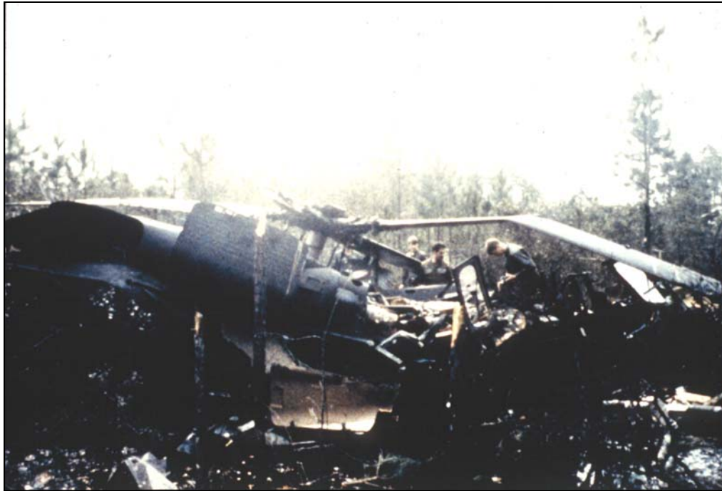
Figure 1. A crash of a UH-60 where the roof completely collapsed, crushing the two rear occupants.
