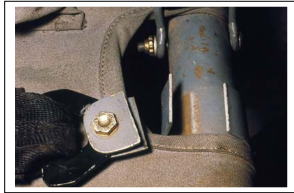
Figure 3. The occupant of this seat was ejected when his lap belt detached from the seat.
