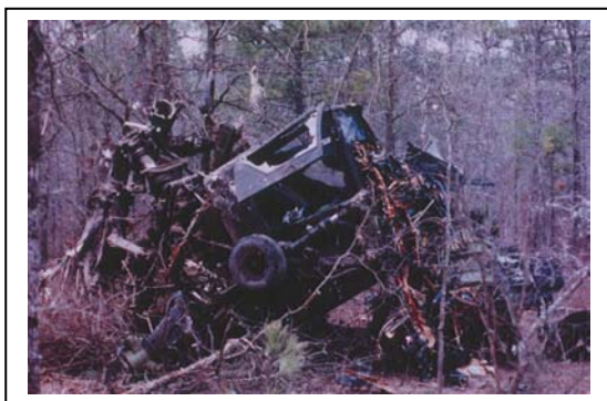
Figure 8. This is a severe crash of an AH-64. The fuel tank was ripped from the helicopter and found some distance from the wreckage.
